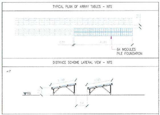
Figure 1-5 PV Arrangement and Mounting Angle
